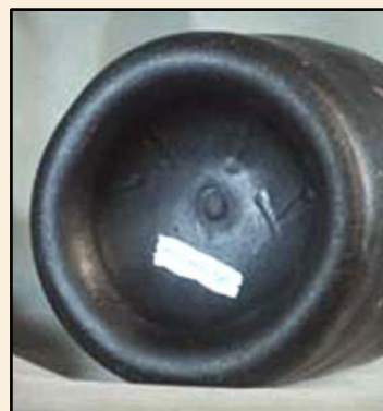
Underside of bottle showing kick-up and small mamelon.
